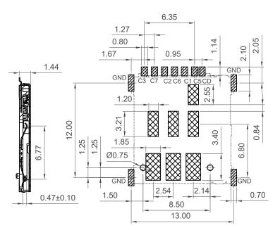
Recommended PCB Layout (Viewed from Component Side - Tolerance:±0.05mm) Solder Area X Keep Out Area C Component Outline
