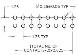
CONNECTOR AND PCB LAYOUT DETAILS ONLY. SEE SHEET 5 FOR TAPE STRIP DETAILS.
