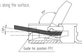
Follow the instructions shown when soldering the connector manually during repair work, etc.
