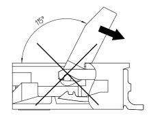
5. Do not pinch or pick the actuator to lift it as shown below. Otherwise it may break. (Do not carry out any operation other than rotating the actuator as shown in 2 above.)
