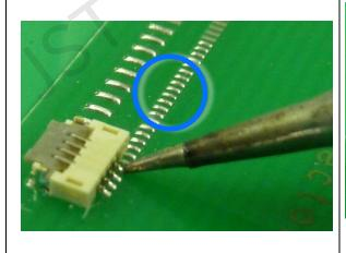
Do not press the soldering iron on the lead part or do not apply an abnormal load, such as lateral one.
