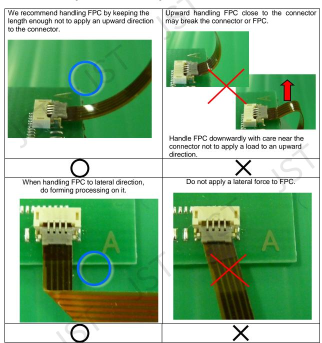
Give attention to using the connector at the place where FPC inserted in the connector moves by the mechanism of the rotating axis of devices or along with the operation of the moveable part, because poor contact may be caused due to fretting corrosion.
