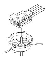
This three circuit connector is used to connect cluster pins (2.3 mm in diameter) to the leads of a motor hermetically sealed in a compressor of a refrigerator or a freezer.
